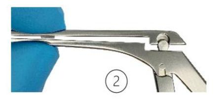
3. Squeeze the upper and lower sliding shafts together lightly so that the guide parts of both shafts (D) engage with each other.
