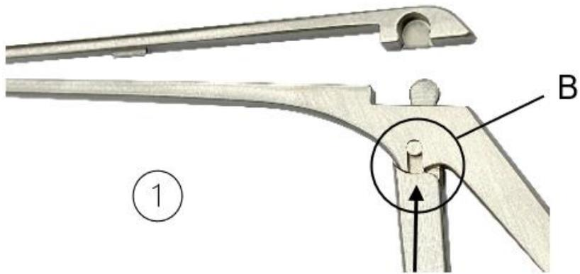
2. Push the upper sliding shaft down and then press it lightly against the lower fixed shaft.
