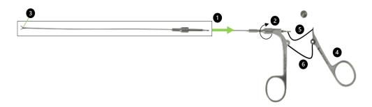
2. Fasten the screw on the handle clockwise.
