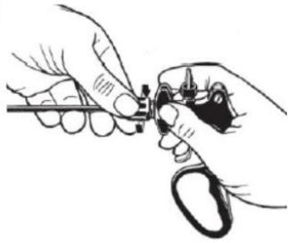
1. Screw the fastening screw nut clockwise onto the threaded socket of the handle and tighten it while holding the rotatable adapter by the handle.
