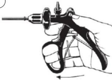
To unscrew the tube, open the instrument or the handle.
